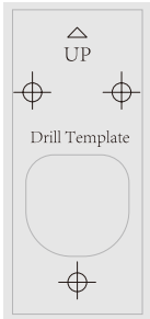
Drill Template for Intercom Panel (x1)
